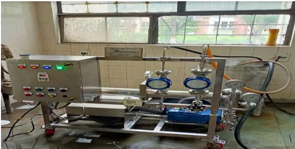
Figure 2: Image of the RO plant used for the concentration of desi buttermilk.
